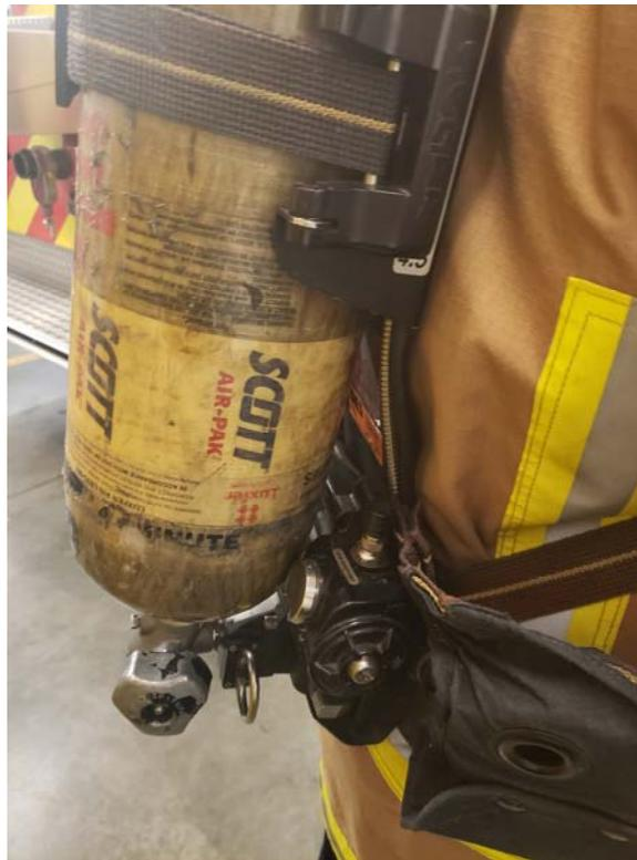
SCBAs provide firefighters with a dedicated air supply when working in environments with smoke or other toxic fumes. The fire district’s SCBAs are from 2007, showing wear and tear, and are past the timeframe for recommended use.
